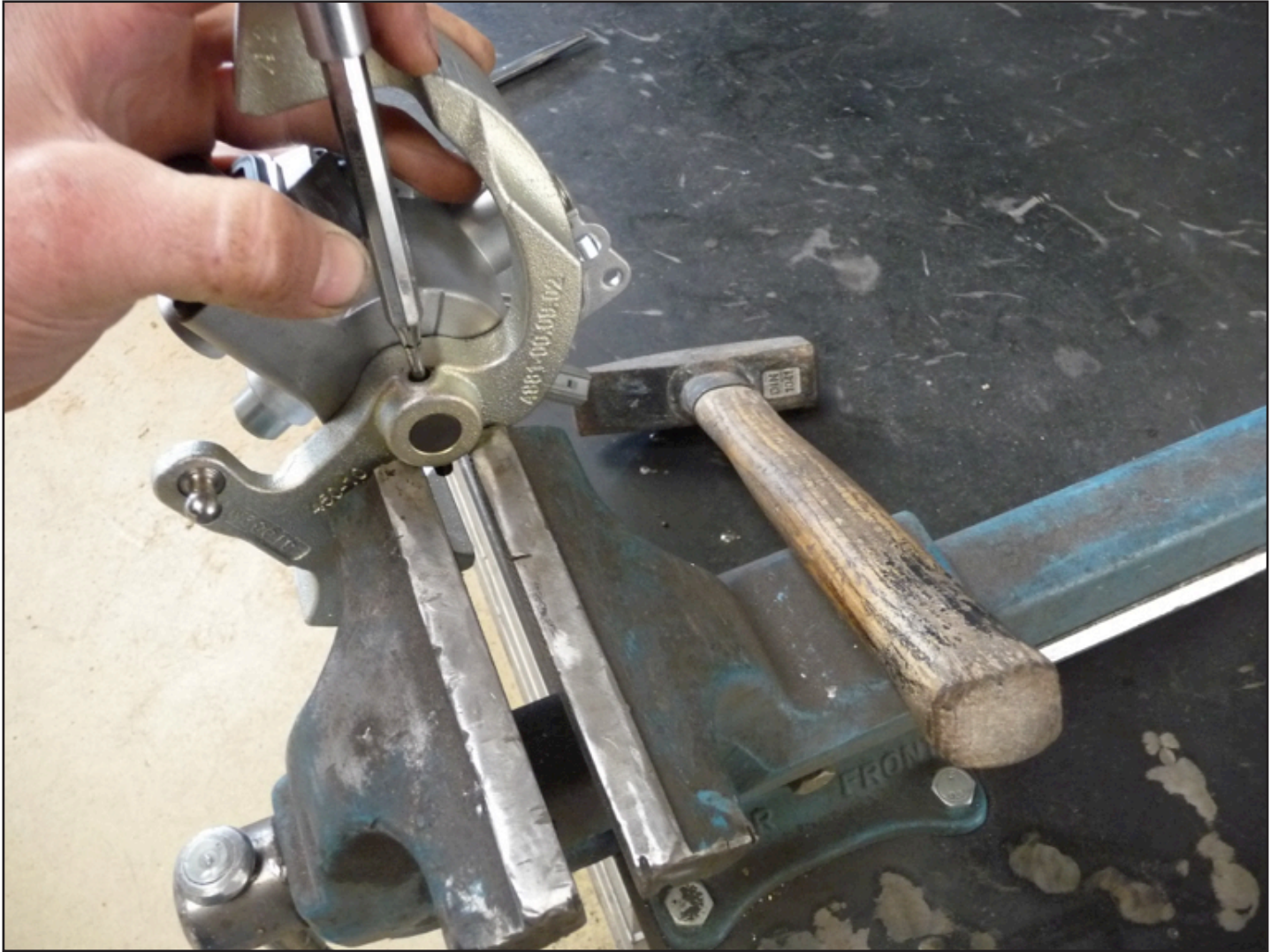
Use a punch to remove the pin from the shifter shaft.
